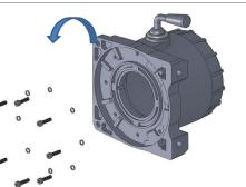
Place the 8 bolts back into the gearbox housing and tighten.
