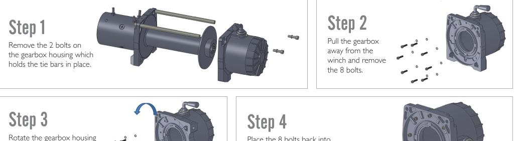
into the desired position. Each bolt hole represents a 45 degree rotation.
